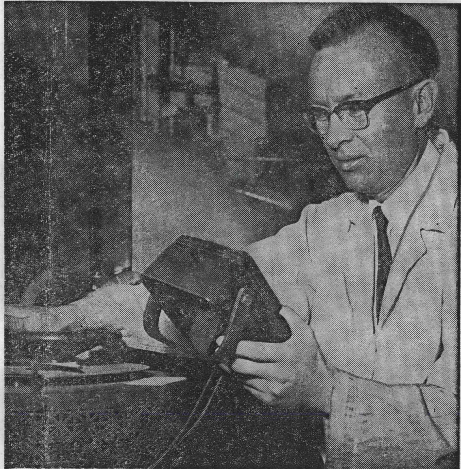
Dr. H. Tracy Hall, director of research at BYU, checks electric meter as he increases the electric current in his high temperature "bomb."
